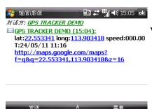
When GPS signals lost, The SMS including the position of latitude and longitude is the positioning that the tracker received GPS signals at last. It may be different with its exact current location, so pay attention to the time included in the SMS.
